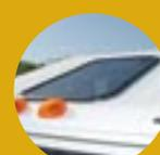
**Roof skylight option** provides additional visibility and light in working situations where overhead sight is important.
